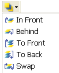
Figure 2.8: You can change the order of entities in your drawing from the Standard Toolbar
