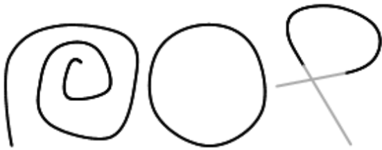
Figure 24.7: Types of contours (Natural, Cyclic, and Tangent respectively)
