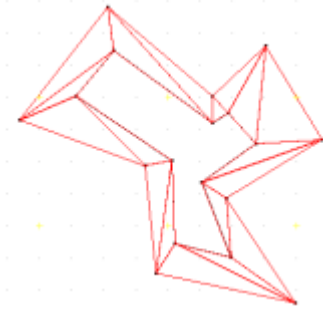
Figure 24.28: Ruled surface between closed concentric polylines
