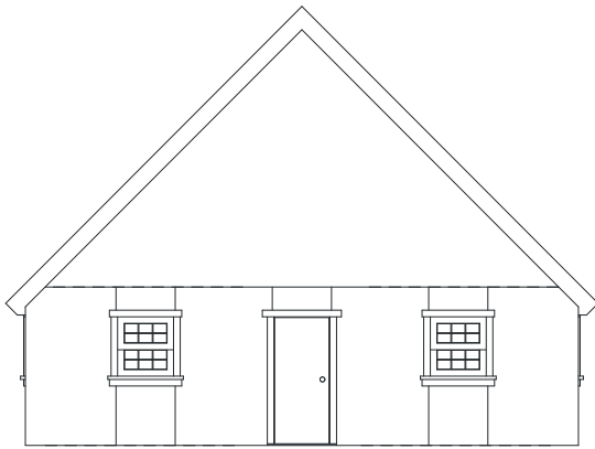
Figure 6.12: The elevation after a hidden line removal
