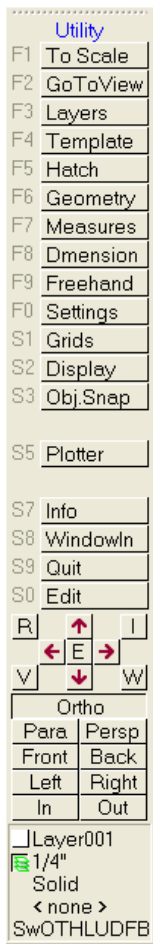
Figure 2.31: The traditional “glued” together menu, complete with buttons, 8-character menu labels, navigation pad, projection pad, and status panel
