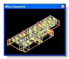
To turn Multi-View Windows on, open your drawing and choose "Toolbars" from the "View" pull-down menu. Place a check mark next to each window that you would like to display. Alternatively, you may open the drawing and press [Ctrl]+[w] on the keyboard to turn on all Multi-View Windows.
