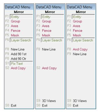
Figure 18.13: 2D Mirror, New 3D Mirror, and 'old' 3D Mirror Menus
