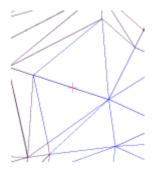
5. Click on the line that separates two adjoining triangles. DataCAD flips the valley.
