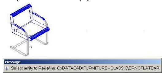
DataCAD has a new "Auto Reload" option, located in the [Ctrl]+[Right-click]/Symbol Tools context menu for symbols. When this option is checked, DataCAD will automatically reload the symbol definition on the hard drive for each instance of the selected symbol every time you open the drawing. This setting is assigned and remembered on a per-symbol (but not per-instance) basis.
