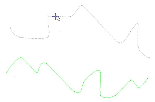
7. Click on the second contour line. DataCAD stretches the ruled surface between the two contour lines. In this example, the distance between divisions was set at 3 inches to produce a very smooth ruled surface.
