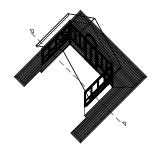
The cut line is a series of dashes; the arrow indicates the view direction
