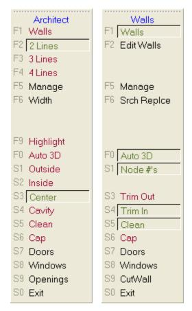
4. Select Manage to display the Wall Type Manager dialog box. Notice that the default is a 2-line wall suitable for an interior wall. If this is what you want, just select OK and begin drawing walls. Otherwise, make sure a checkmark appears in the Display External Types box and continue to refine your choices.
