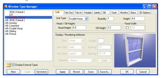
3. Refine the window properties by using the options in the various tab sections of the Window Type Manager.
