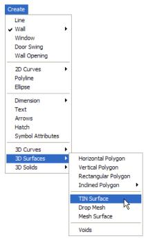
4. Select Area, click above the top left contour, draw the rubber band around the set of contours, and click to end the box. DataCAD generates the TIN model.
