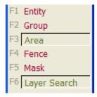
Mask lets you define selection filters on the fly. The Mask filters you can activate, and set are Entity, Color, Line Type, and Weight. Previously-defined masks are retained for subsequent editing operations.
