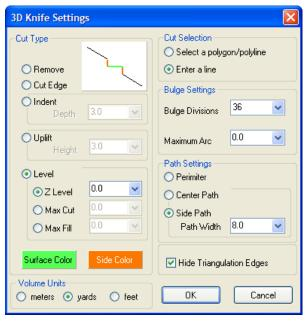
5. Make selections from the Cut Type options. The options you activate in Cut Type portion of this dialog box affect the number of settings you can control in other parts of the 3D Knife Settings dialog box. If an option is gray in the dialog box, it is unavailable.
