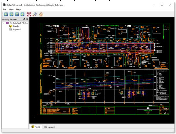
When you import a DWG file that includes Paper Space Layouts, DataCAD will display a new option, Include Paper Space, on the DWG Import Entity Assignments dialog. Check this option to include Paper Space Layouts and any Paper Space-specific entities from the DWG file during import. If the DWG file does not include any Paper Space Layouts, the Include Paper Space option will be greyed out.
