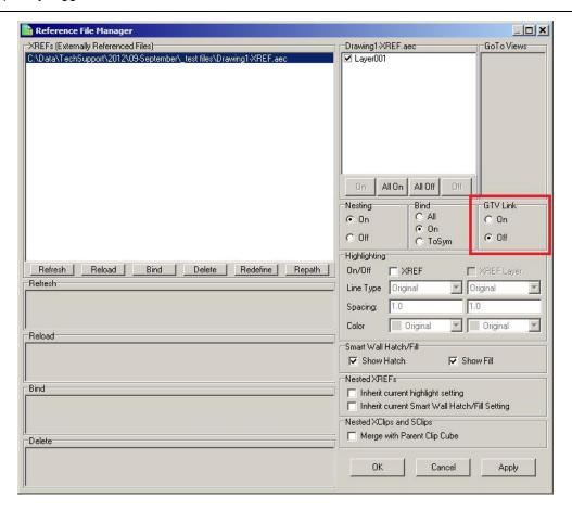
The GTV Link feature now supports per-XREF highlighting in addition to the per-XREF-layer highlighting that was previously supported. Using this feature, you can insert an XREF and assign highlight color, line type and line spacing, and then save a GoTo View in the host drawing. You can then assign different (or no) highlight color, line type and spacing, save another GoTo View in the host drawing, and DataCAD will remember these settings when switching between GoTo Views.
