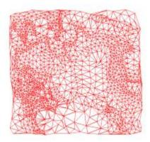
The surveyor may have inadvertently duplicated points in the data file. This could result in a TIN model that takes up more storage space than necessary on your computer. To control the size of your file, you can eliminate duplicate points before you generate the TIN model.
