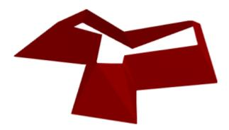
Once you have created a ruled surface between two contour lines, two polylines, or two concentric closed polylines, you can use 3D Knife functions to cut out, uplift, or indent irregular shapes or areas. Just treat the ruled surface as if it were a TIN model.
