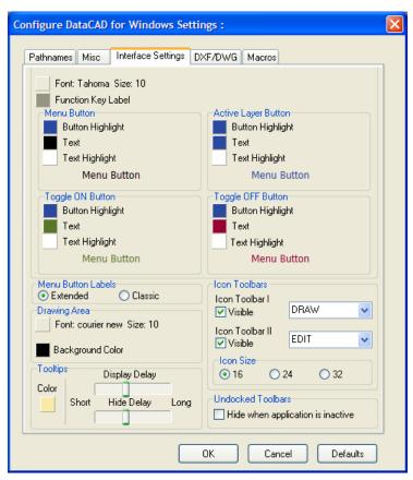
The Default Toolbar section allows you to configure icon toolbars 1 and 2 based on selections from pull-down menus
