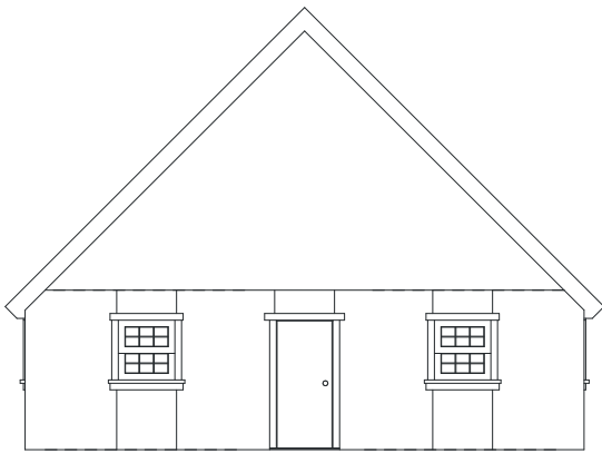
Figure 6.12: The elevation after a hidden line removal
