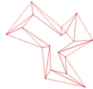
Figure 24.28: Ruled surface between closed concentric polylines
