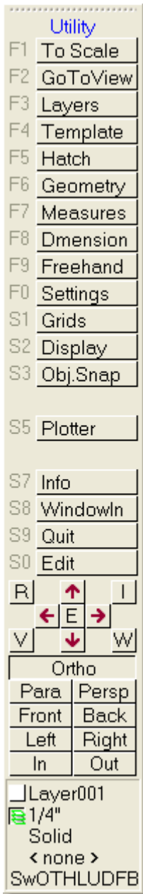
Figure 2.31: The traditional “glued” together menu, complete with buttons, 8-character menu labels, navigation pad, projection pad, and status panel
