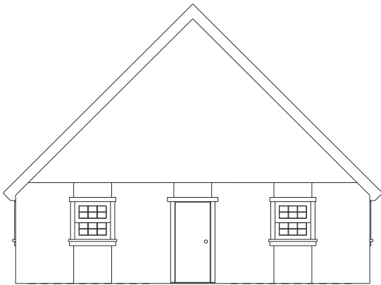
Figure 6.12: The elevation after a hidden line removal
