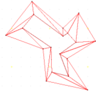
Figure 24.28: Ruled surface between closed concentric polylines
