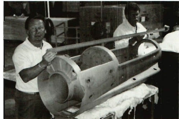
Bill and Tom Schrey measuring the 64-inch pattern cast in non-soluble wax.
