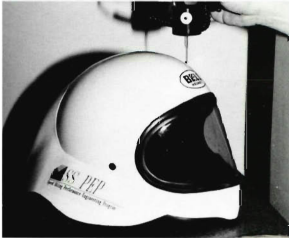
Physical prototype of aerodynamic safety helmet for speed skiing.
