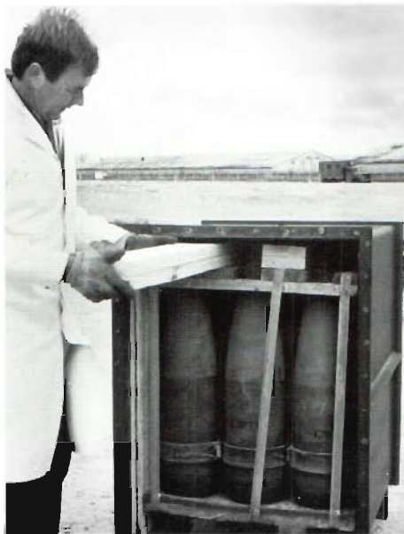
Jerome H. Krohn, Acting Chief of the Validation Engineering Division of the Logistics Engineering Office of the U.S. Army, places wooden, vertical-restraint dunnage into a Secondary Steel Container loaded with inert, 8-inch, separate-loading projectiles during a test at the U.S. Army Defense Ammunition Center and School, Savanna, Illinois.
