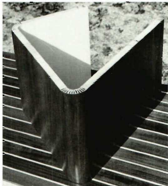
A sample of a significant advance in the technology of building boats: Decolite ™ composite panel bent at 60-degree and 90-degree angles, with 2-inch outside radii, epoxied with teak veneer using the vacuum-bagging technique, produced by Tim Allen.
