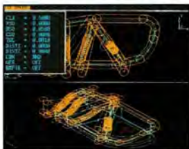
Cutting Edge features simultaneously active viewpoints (tool path shown here).
