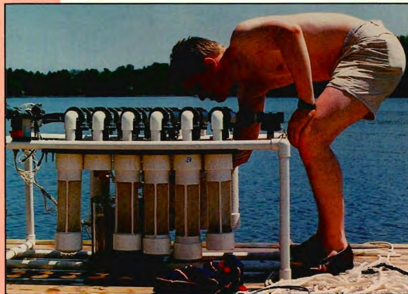
Getting the REPPS (REmote Programmable Plankton Sampler) ready for submersion.
