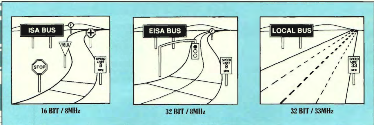
The Local Bus provides a wider roadway and operates at CPU speeds. Optimal Local Bus Architecture allows speed critical peripherals- graphics, disk and network -to interface directly with the Local Bus moving data at CPU speeds. Illustration -courtesy of Appium Technology, Inc.
