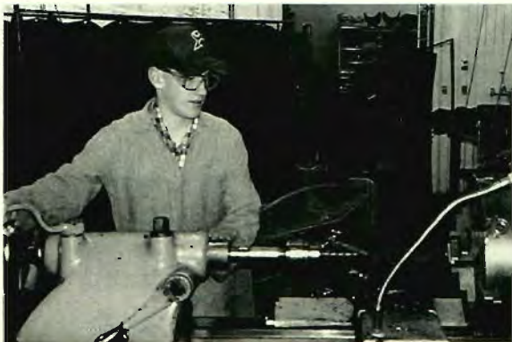
Student, Andrew Stewart, cutting a steel taper and hinge pin in Selkirk's shop.
