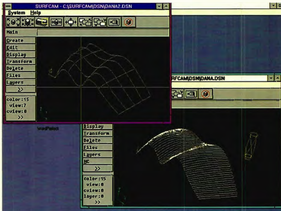
MACHINABLE SURFACE FROM CADKEY SPLINE MESH IN SURFCAM FOR WINDOWS.
