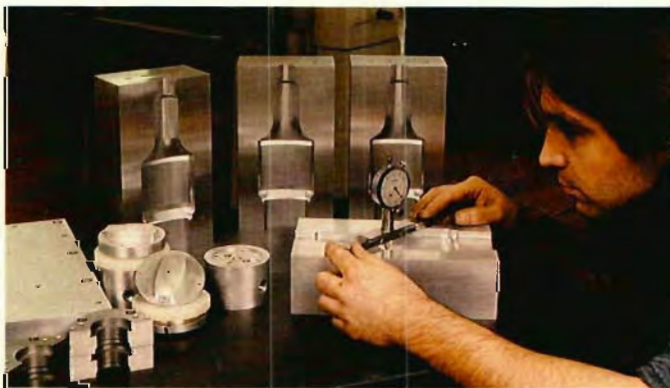
Components to be assembled into the finished mold, including cavities, mounting plates and bottom plugs; technician checking cavity depth with a dial depth gauge.
