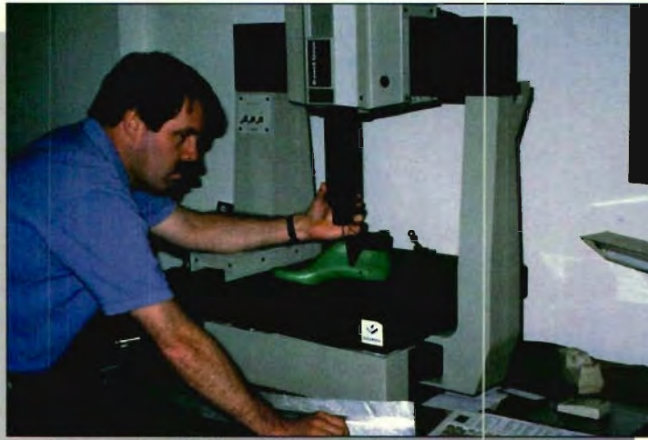
Using CADDInspector with a Brown & Sharpe coordinate measuring machine.
