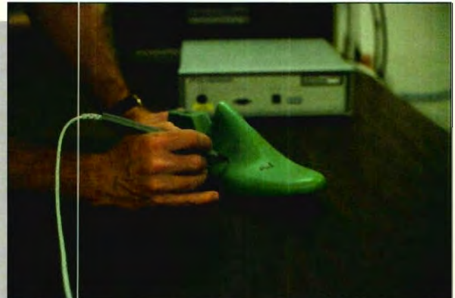
Digitizing a polycarbonate last with a Polhemus ISOTRAK II.
