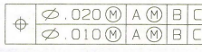
Figure 2: Composite Positional Tolerance With Additional Datum References in the Feature Locating Control Frame
