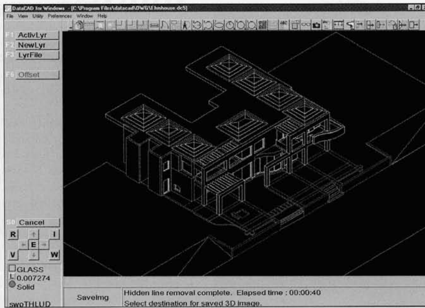
Figure 5. Hidden line views can be displayed easily, and then saved in a 2D representation to another layer in the current drawing for further editing.
